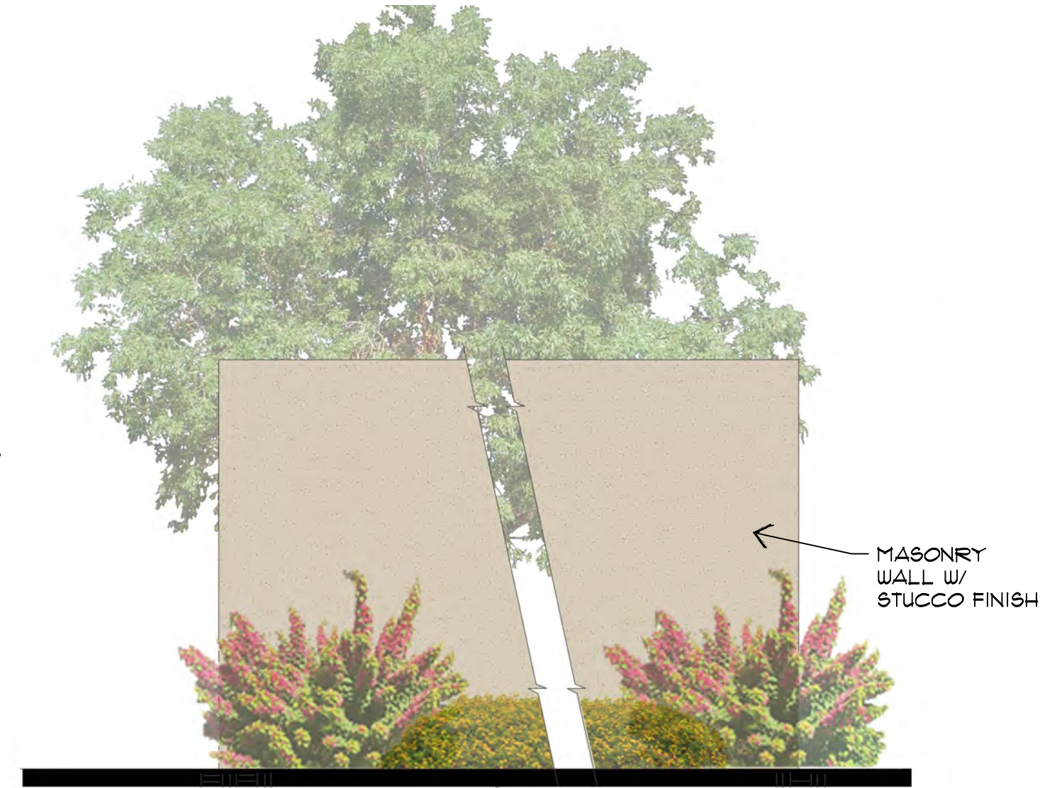
3 PERIMETER MASONRY WALL SCALE: NT8
